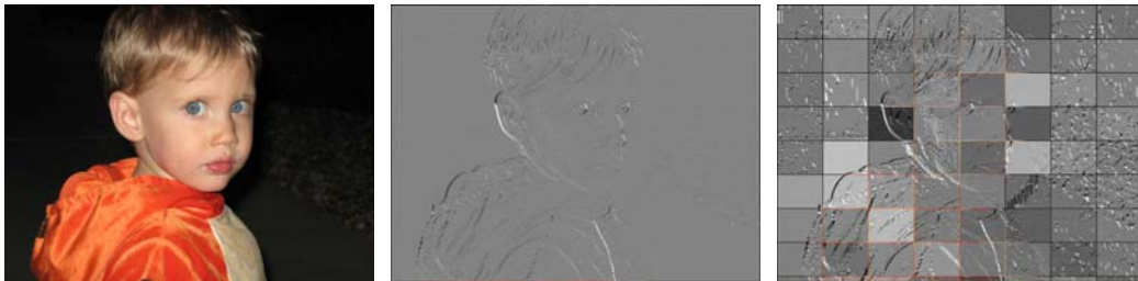
Figure 4: Sobel Edge Detection Results. Left: Original Image, Center: Single processor example, Right: Map/Reduce using the Blob Detection Input Format and Record Reader.
