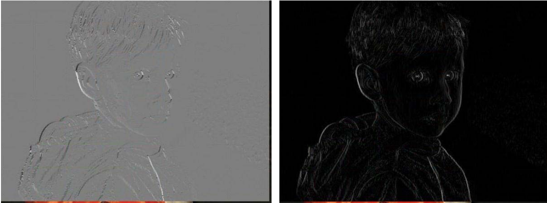
Figure 7: Comparison of the correct implementation of the Sobel Edge Detection algorithm (right), with our initial implementation of the algorithm (left)
